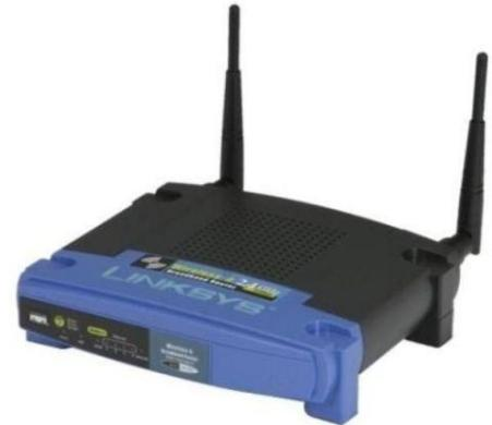
HSMM-MESH is a digital communication mode that lets computers communicate using WiFi networking hardware on amateur-radio bands. The scheme that the mode provides is not limited to single point-to-point links: equipment automatically manages the routes of the mesh network, rerouting as necessary around broken network links. So this sounds great, but . . . why do I care?
