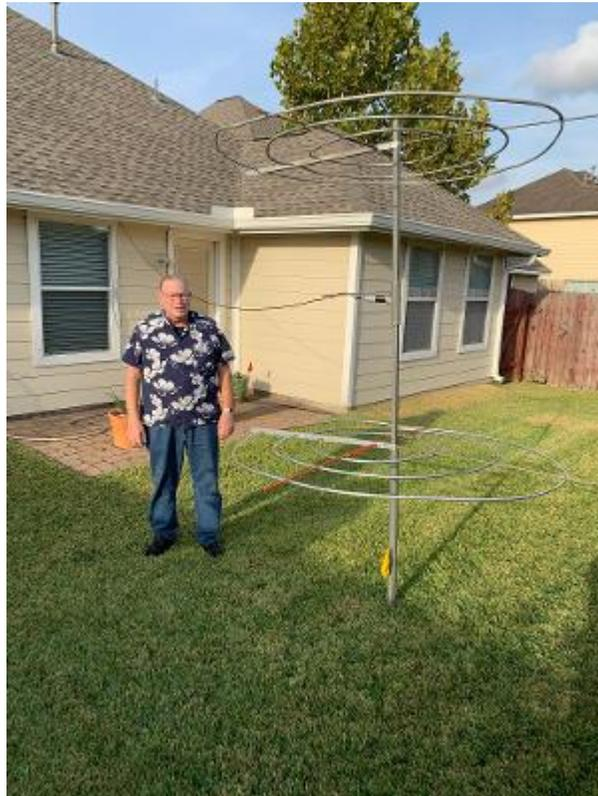
Me and my "ZR-3 style" homemade vertical dipole antenna
